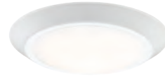
VRG1608W 1.25" H x 7.75" W x 7.75" D Finish: White Lustre Integrated LED Lumens: Delivered 975 | Initial 1300 Kelvin 3000, CRI 90 ETL Listed Location: Damp
