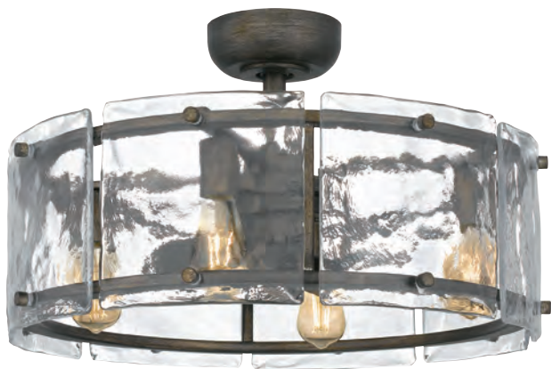
FTS3124MM | FAN LIGHT 9.75" H x 24" W x 24" D 4 - 8W LED Medium Base (Included) Kelvin 2400, CRI 90 Hanging Height Max: 23.00 ETL Listed Location: Damp
